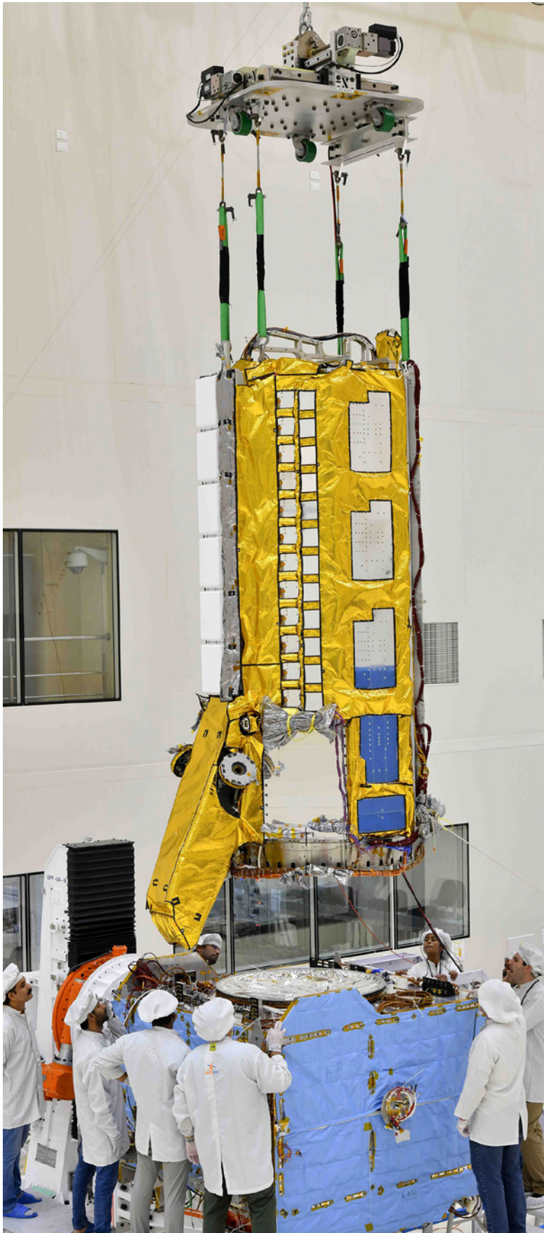
Photo 2. In June, engineers used a crane to align NISAR's radar instrument payload—seen partially wrapped in gold-colored thermal blanketing—with the satellite's spacecraft bus, which is inside the blue blanketing. Photo credit: VDOS-URSC
