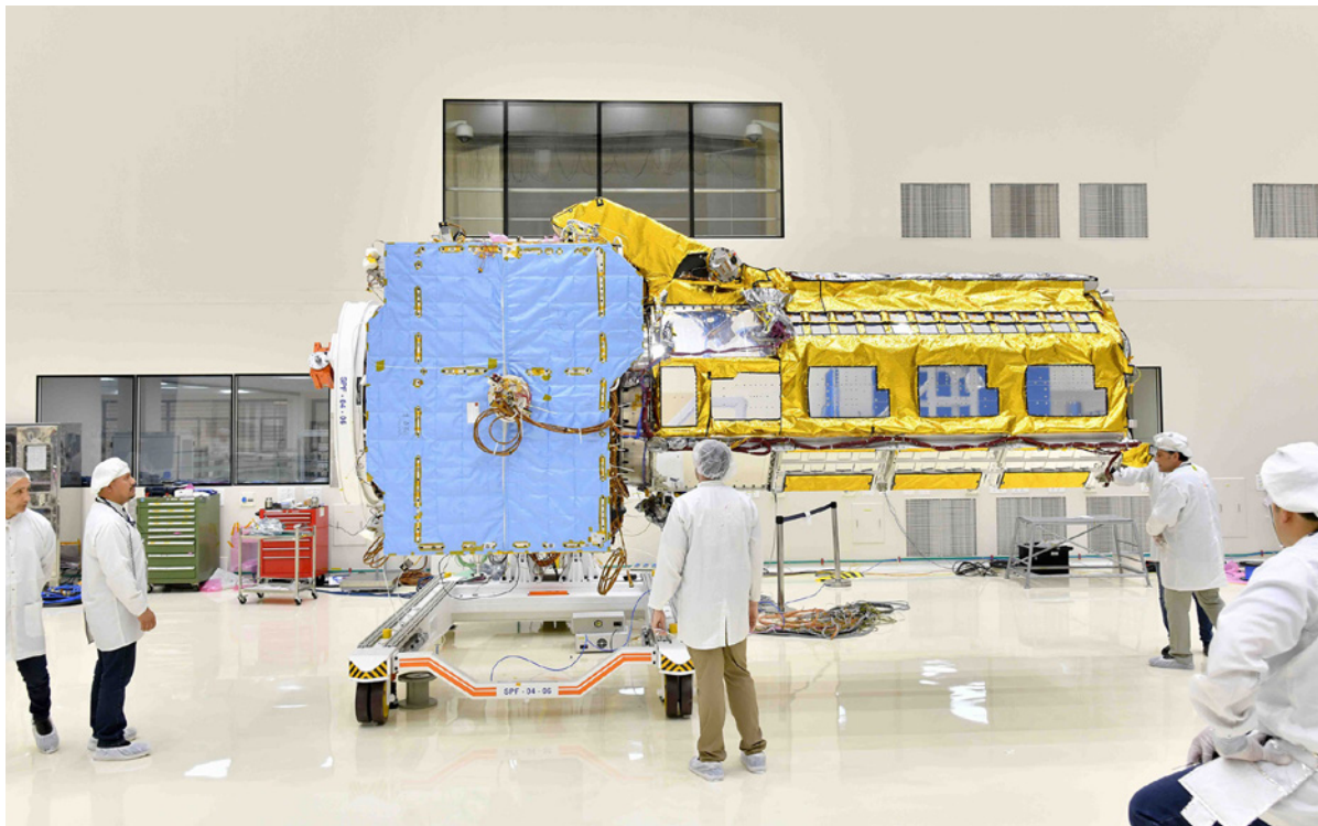
Photo 1. Engineers joined the two main components of NISAR—the spacecraft bus and the radar instrument payload—in an ISRO clean room in Bengaluru, India, in June. The payload arrived from NASA's Jet Propulsion Laboratory in Southern California in March, while the bus was built at the ISRO facility. Photo credit: VDOS-URSC
